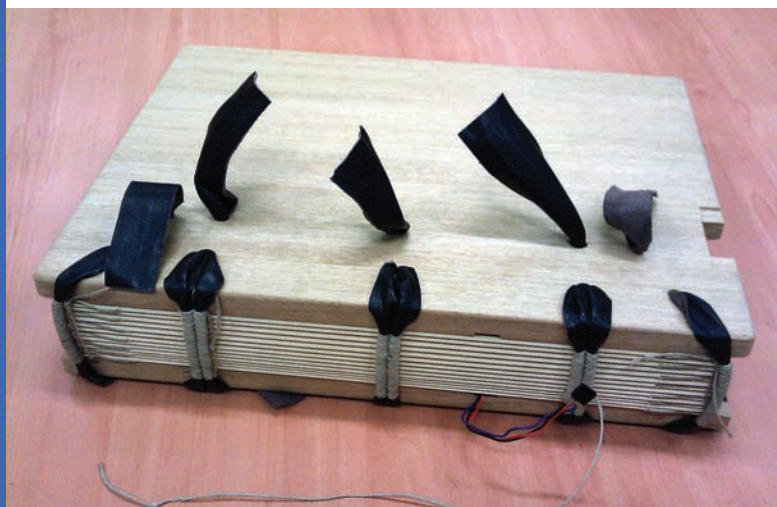
FIG.8 E 8A TESTING PROTOTYPE FOR THE AUGMENTED BOOK
