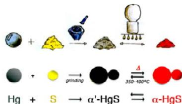
Figure 2. Reaction scheme for vermilion synthesis.
