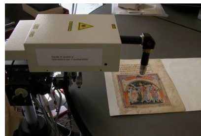
FIG.18 ANALYSIS OF MINIATURES BY RAMAN SPECTROSCOPY
